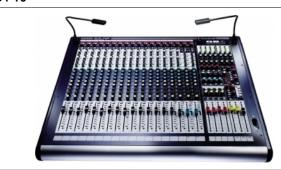
16 mono inputs. GB30 mic preamps with phantom power, phase reverse and HPF filter. 4-band EQ. 4-segment LED meters on every channel. Direct outputs on every channel (pre/post selectable). Two stereo channels. 8 aux sends. 4 sub groups. 4 mute groups. 100mm faders. Dual FOH/monitor modes. 7x4 output matrix. L, R and C outputs. Record out with limiter. Internal PSU with external option.
