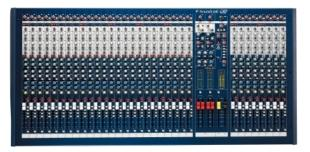
32 channel 4-bus live sound console. GB30 preamps and 4-band EQ with semi-parametric mids. 6 aux sends configrable in pairs as pre- or post-fade for monitor or effects operation. 100mm faders. Comprehensive master section with talkback, two stereo returns and 12-segment group and master LED meters.
