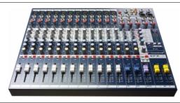
EFX series have the same features as the EPM series but with the addition of an on-board 24-bit effects processor using the same AudioDNA chip as many of the Lexicon effects units. 12/2 frame size.
