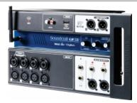
12-input Ui Series mixer. Four XLR combo mic/line inputs, four XLR mic inputs, two channels of Hi-Z instrument inputs, stereo RCA line input. 2 channel USB media player. Two XLR Aux outputs, two 1/4" headphone outputs plus stereo XLR and 1/4" main outputs.
