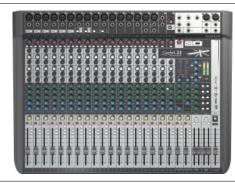
High-performance 22-input small format analogue mixer with onboard effects and multi-track USB interface. 22 channels. 16 Ghost mic preamps, 4-band Sapphyre EQ. 8 dbx limiters on input channels. 5 auxes. 4 mono/2 stereo subgroups. 24-in/22-out USB interface. 100mm faders. Dual-engine Lexicon effects.
