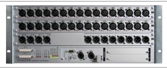
Compact stagebox designed for use with the Vi and Si Series consoles including the Si Compact. 8 GPIO inputs and outputs for control over/from external equipment. Two expansion slots take D21m cards. Connection to the host is via Cat5 or optical MADI. Configured as 32 analogue in, 8 analogue out, 8 AES out. Cat5 MADI connection
