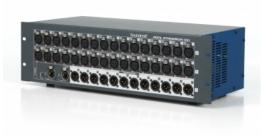
Remote stagebox for Soundcraft Si series consoles. 32 Studer-designed remote controlled mic preamps and AD converters. 12 XLR analogue line level outputs. Dual MADI RJ45/Cat5 connectivity, for 100M runs between stage and mixing console. 3U Rack mount design.
