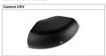
Unique contemporary curved design, combinable into 180°, 270° or 360° round arc clusters. Selectable 70/100V or 4 ohm. 80Hz-20kHz frequency response. 75W continuous. 89dB sensitivity. 105° horizontal, 80° vertical. Indoor/outdoor capable (IP34). Wall mount bracket included. Black or White.
