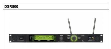
The DSR800 reference two-channel digital wireless receiver provides an ultra-wide bandwidth of up to 150MHz for reliable operation with the flexibility to meet the needs of a wide range of applications. It is designed to work with the versatile DHT800 handheld transmitter, which offers interchangeable microphone capsules, and the DPT800 body-pack transmitter, for line- and microphone signals.
