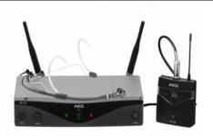
Single channel wireless system with assignable frequency selection. Compatible with the CU400 charging station and AKG's external antenna components. Set consists of SR420 receiver, power supply, PT420 belt-pack transmitter and C555L head worn microphone. Band U1 for Channel 38, band D for licence-free ISM/Channel 70.
